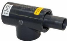
**Eductors** are constructed of PVC that deliver the correct brine concentration to the condensate polisher resin. These hydraulic injectors are pressure compensating and produce 10-16% dilute brine concentrations to the polisher bed for proper ion exchange. Pumped brine systems and brine silos are available.
