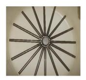
**Underdrain** The radial hub underdrain uses high quality PVC pipe and fittings, delivering high performance standards. The .010" PVC slotted laterals are installed to utilize the entire bed area minimizing channeling during low flow. This design provides high flow rates, reliability and quality assurance. **Lakeside's four point header inlet baffle on 48" and larger vessels increases even flow distribution.**
